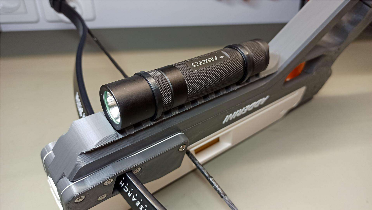
You can also mount the Convoy S2+ flashlight directly to the cocking lever. Print the appropriate part and use 2 zip ties.
